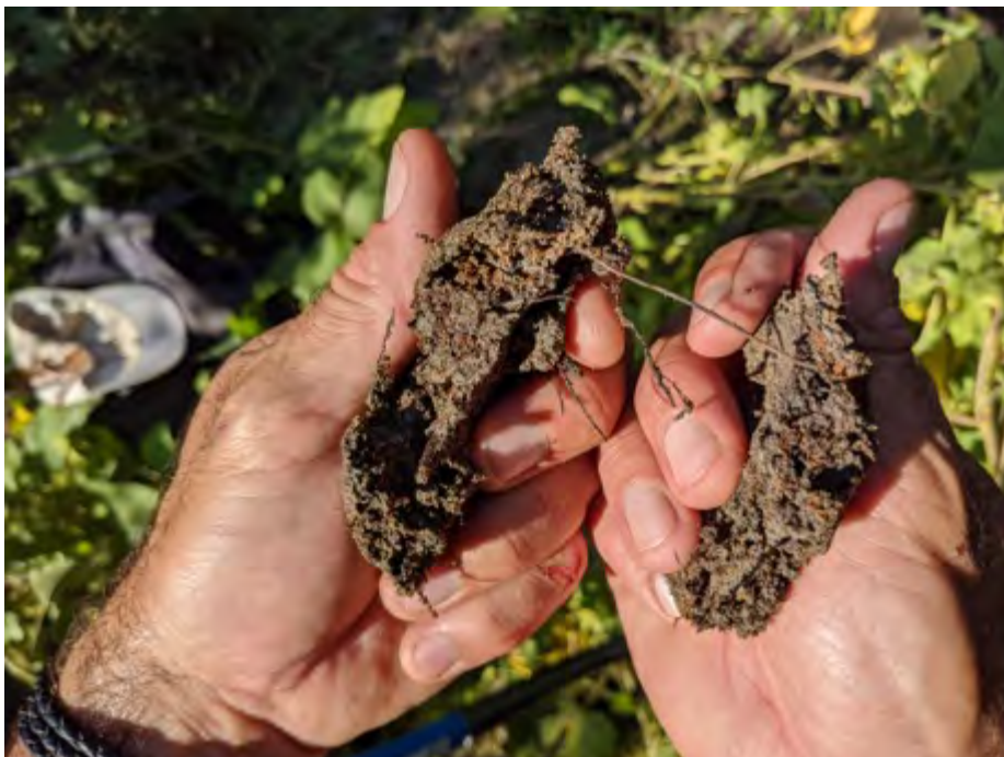
Photo 6: A representative photo showing hydric soils from a sampling pit in the southern willow scrub habitat. Note the prominent redox concentrations in the soil matrix, visible as rusty-colored plotches and as pore linings.
